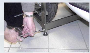
Adjust the position of the tool to that all the cursors are in contact with the wheel, and not with the tyre
