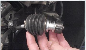
Tighten the nut fastening the joint onto the suspension to the specified torque
