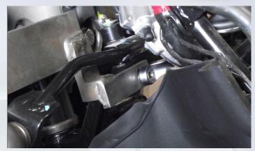
Fasten the steering orientation tool to the parallelogram with the original screws
