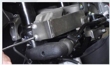
Reposition the vehicle in the tool and repeat measurement of toe-in/toe-out. Check whether the error is relative to the suspension on both wheels or on just one wheel
