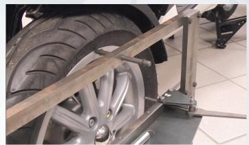
Using the camber measurement cursors as reference, correct the vertical position of the vehicle by adjusting the shock absorber lock system
